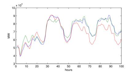
Figure 3: Cutout of three arbitrary load paths generated with SMaPS
